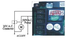
Figure 3-8 Wiring of Booster Pump on Inlet
