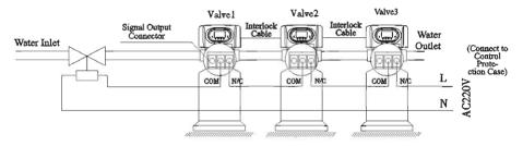
Figure 3-4 Wiring of Solenoid Vale in Inlet
