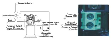
Figure 3-10 Wiring of Pressure Relief Output Figure 3-11 Wiring of Remote Input
